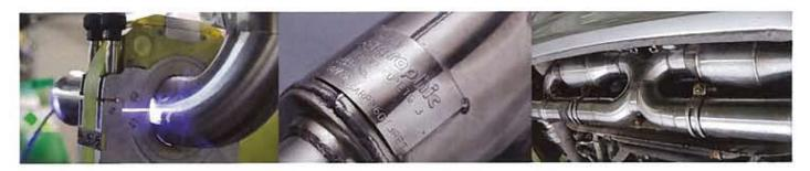
Above left to right: Tubes are argon filled during welding. All important iD plate, complete with TUV number. Jumping ahead somewhat, but exhaust in situ. It's a quality piece of kit. Below: Our exhaust fits the set-up jig like a glove
