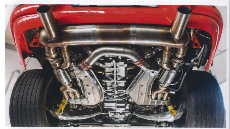
outlet. Strengthened brackets, as well as the olive-and-slide system ensure an exact adjustment, which guarantees a stressfree installation.
